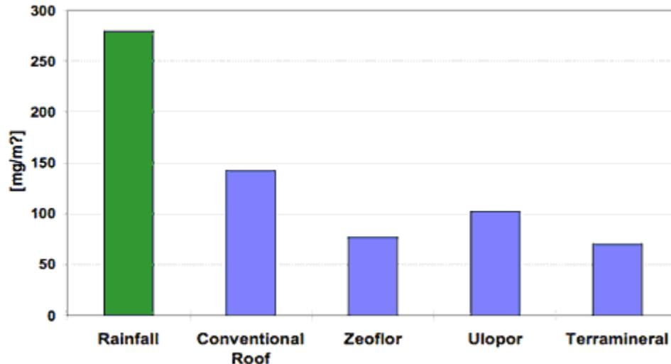
**Illustration 10: Discharge of o-PO<sub>4</sub>-P from 8/7-11/3/97 and from 1/8 –1/21/98**
