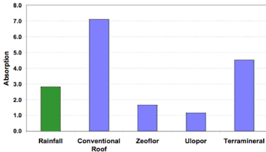
**Illustration 6: Turbidity of runoff, measured at 420 nm, from the tested substrates between 8/7/97 and 1/21/98**
